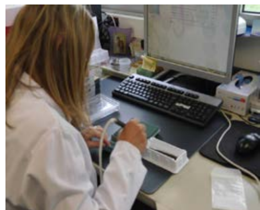
A seed analyst using the vacuum pump to set up small seeds for a germination test.
